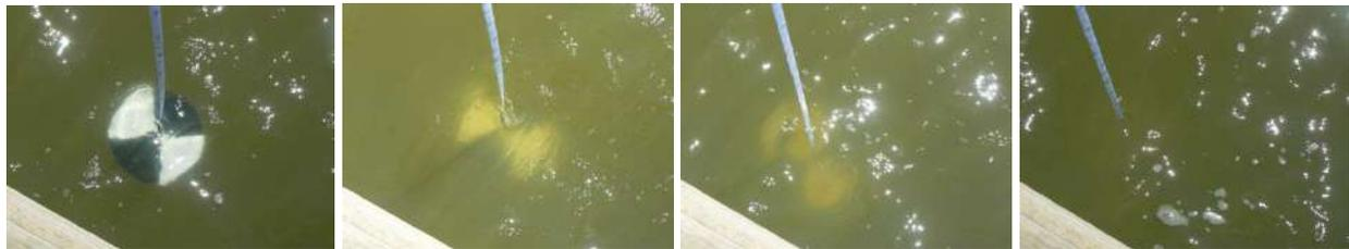
3. Pull the disk up carefully so that the pegs do not move. The Secchi depth is the distance between the two pegs (i.e. steps 1 and 2), recorded to the nearest centimetre.
