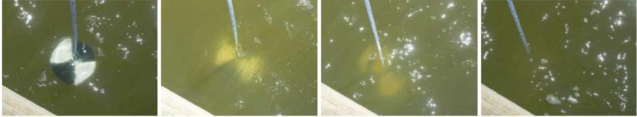
2. Place a peg on the rope/ tape measure at the water's surface when the disk disappears from view. This is the Secchi depth (record it to the nearest centimetre).
