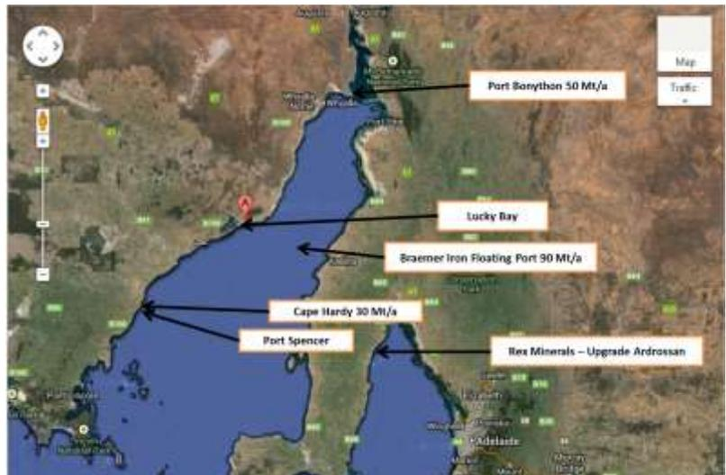
At Lucky Bay, IronClad plans to cart crushed iron from Wilchery Hill mine to Lucky Bay in road train trucks, then to 70 M long barges for trans-shipment, then loading onto 70K tonne panama export vessels 9km offshore.
